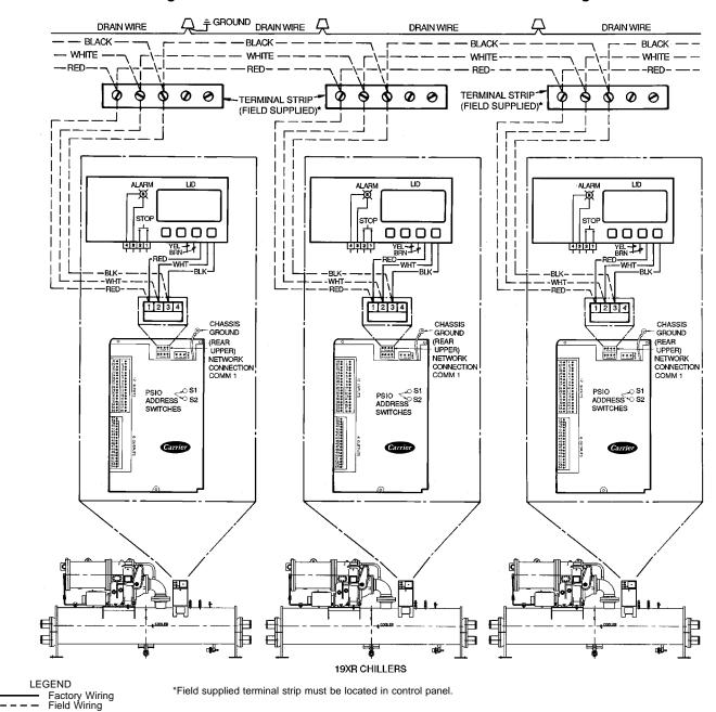
Fig. 25 — COMM1 CCN Communication Wiring For Multiple Chillers (Typical)
